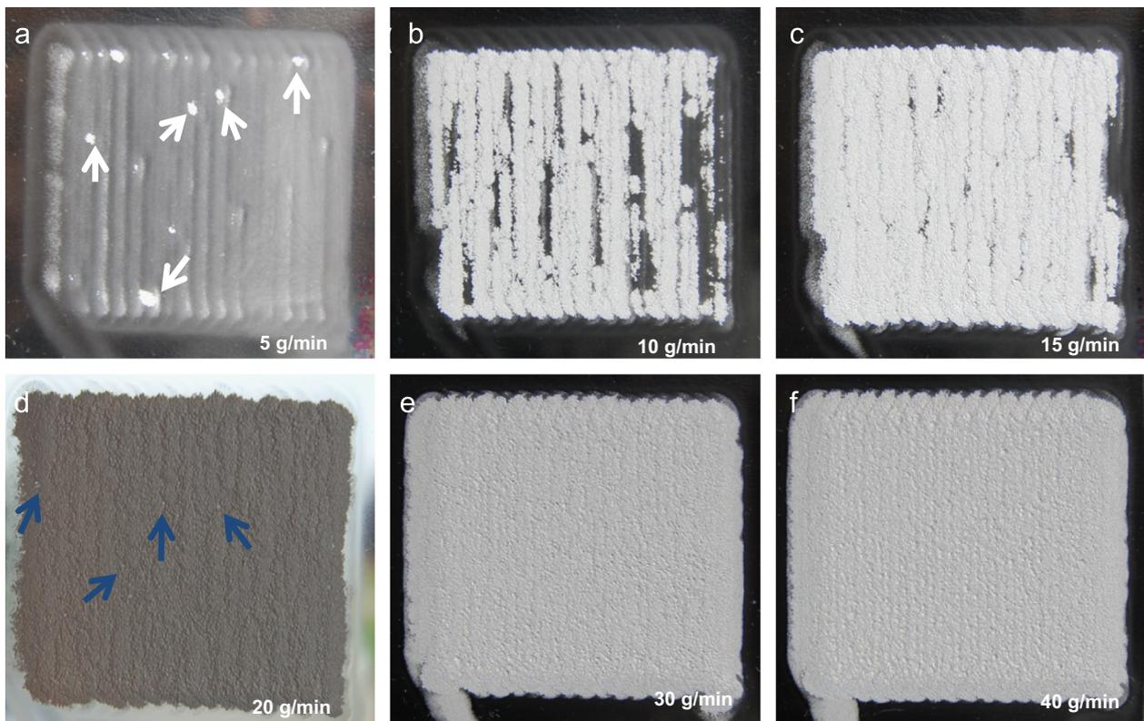
Fig. 2. Surface morphology of Al deposition on Lexan at different powder feeding rates. (For interpretation of the references to color in this figure, the reader is referred to the web version of this article.)
