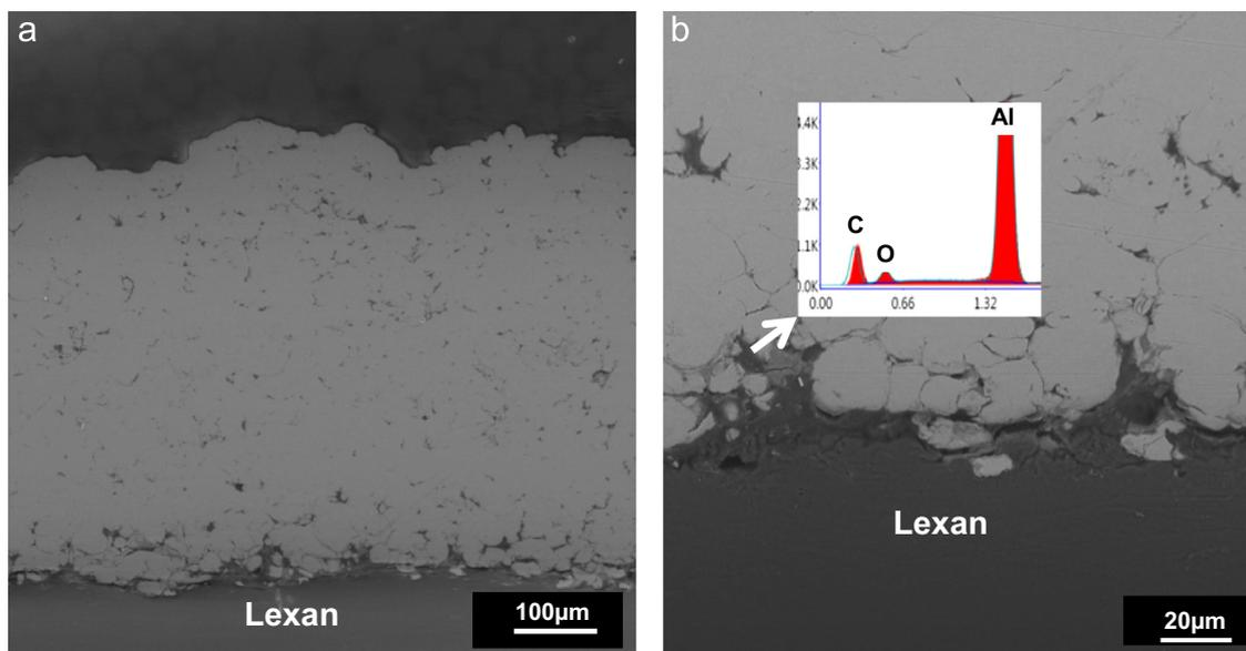
Fig. 4. Microstructures of the coating and interface achieved at 40 g/min powder feeding rate.
