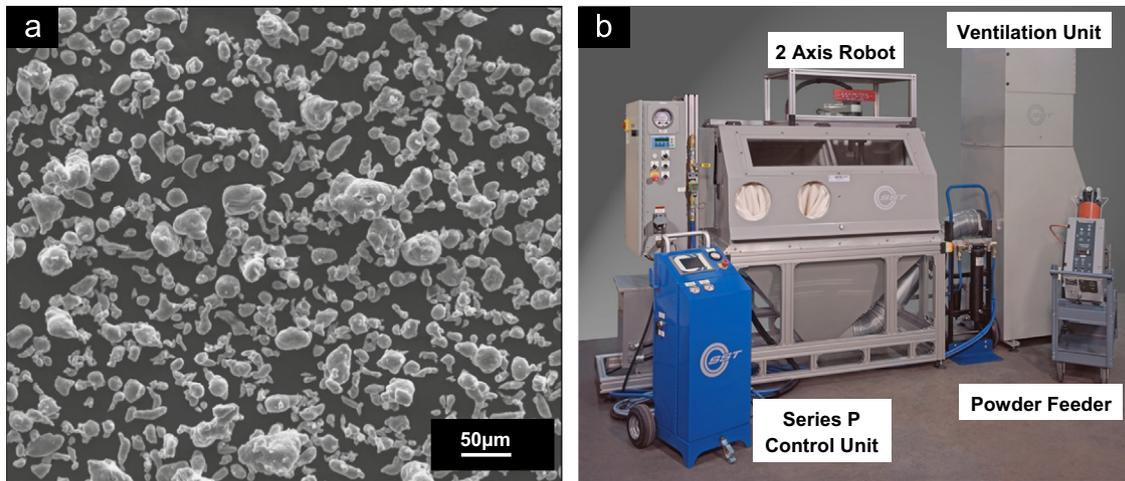
Fig. 1. SST-A5001 SEM morphology (a) and Supersonic Spray Technologies Series P cold spray system (b).
