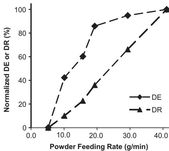
Fig. 3. Normalized deposition efficiency and deposition rate at different powder feeding rates.
